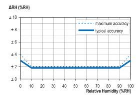
Typical accuracy of relative humidity measurements given in %RH for temperatures 0 to  $80^{\circ}\text{C}$ .
