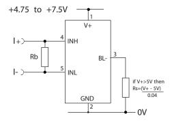
Measuring a current from a circuit which is floating with respect to the DPM's supply, i.e. the current and the meter's power supply are isolated from each other.
