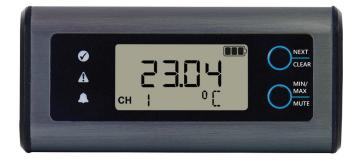
Monitor the environment you live and work in with the EasyLog EL-SIE-6+. Configuration is simple, with no software to install on your PC or Mac – just connect the logger with a USB cable, and use your standard web browser to configure the device for logging. You don't even need internet access to set up and use the EL-SIE-6+, it really couldn't be easier.
