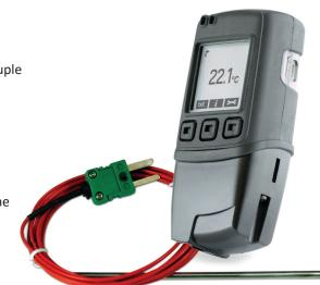
This standalone data logger measures and stores more than 250,000 temperature readings from a K, J or T-type thermocouple at a resolution of 0.1°C (0.2°F). It comes supplied with a K-type thermocouple capable of measuring from 0 to 200°C (32 to 392°F).
