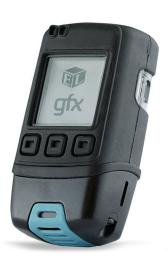
This stand-alone data logger measures and stores over 250,000 temperature and humidity readings over a -30 to 80°C (-22 to 176°F) and 0 to 100%RH range at a resolution of 0.1°C (0.2°F) and 0.1%RH.
