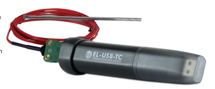
This standalone data logger measures and stores more than 32,000 temperature readings from a J, K or T-type thermocouple at a resolution of 0.5°C (1°F). It comes supplied with a K-type thermocouple capable of measuring from 0 to +200°C (+32 to +392°F).
