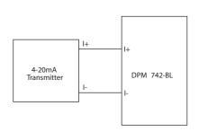
Measuring a 4-20mA loop current.
