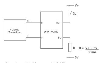
Measuring a 4-20mA loop current with LED Backlighting switched on.
