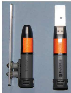
Modified mounting allows the logger to attach directly to the mine wall
