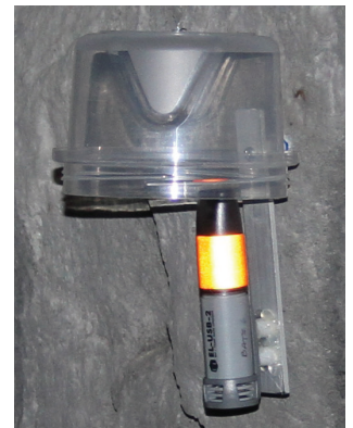
Modified mounting allows the logger to attach directly to the mine wall
