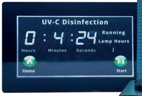
Evergreen UV's EDU uses the smaller, 4.3" PanelPilotAce model (a larger 7" version is available) which Sears claims is the "most integral part" of the EDU as a whole, not least because it allows users to set a delayed start time, run time, log data, and get notifications of when the EDU's UV lamps need to be replaced.
